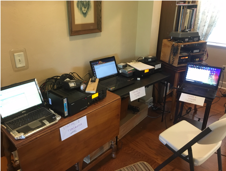
Three radio stations with computers and pactor modems. Far left is Station #1 (“Transmitter”) On the black table is Station #2 (“Intended recipient”) and at the far right is Station #3 (“Snooping Station”)
